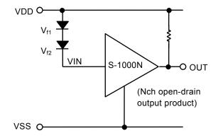
Detection voltage =  $V_{f1}+V_{f2}+(-V_{DET})$
