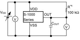
\*1. R is unnecessary for CMOS output products.
