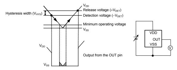
Remark For values of V<sub>DD</sub> less than minimum operating voltage, values of OUT terminal output is free in the shaded region.
