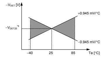
\*1.  $-V_{DET25}$  is an actual detection voltage value at 25°C.
