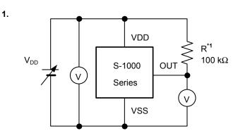
1. R is unnecessary for CMOS output products.
