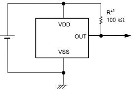
\*1. R is unnecessary for CMOS output products.
