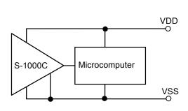
Figure 24 Reset circuit example(S-1000C)
