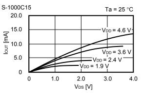
8. Pch transistor output current (IOUT)
