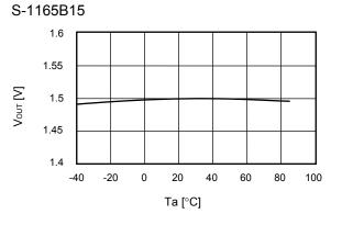
(5) Output voltage vs. Ambient temperature
