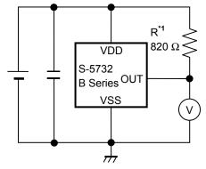
\*1. Resistor (R) is unnecessary for Nch driver + built-in pull-up resistor product.
