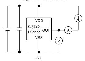
Figure 6 Test Circuit 2
