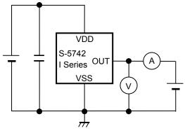
Figure 7 Test Circuit 3
