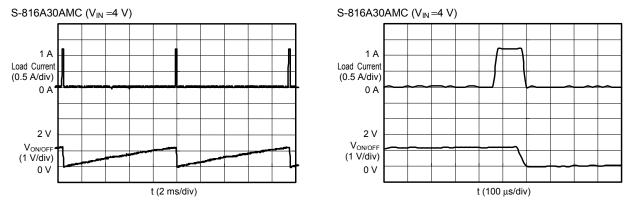
Figure 12 Output Current Waveforms during Intermittent Operation Prompted by Load Short-Circuiting
