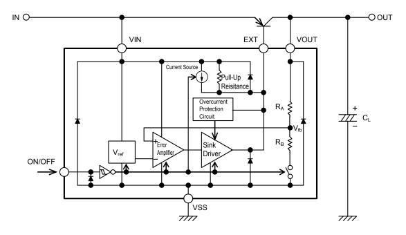
**Remark** The diode inside the IC is a parasitic diode.
