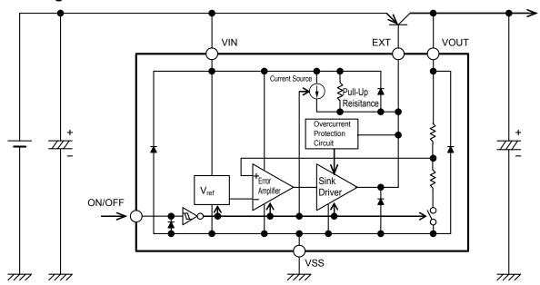
**Remark 1.** To ensure you power cutoff of the external transistor when the device is powered down, the EXT output is pulled up to  $V_{IN}$  by a pull-up resistance (approx. 0.5 M $\Omega$ ) inside the IC.
