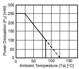
Figure 3 Power Dissipation of Package
