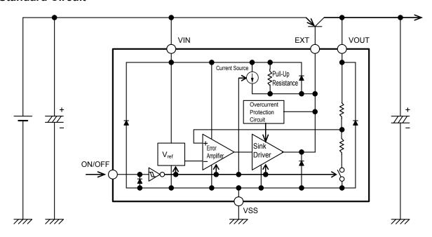
Remark The diode inside the IC is a parasitic diode.
