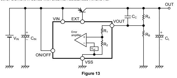
The S-816 Series has an internal impedance resulting from  $R_1$  and  $R_2$  between the VOUT and the VSS pin, as shown in **Figure 13**. Therefore, the influence of the internal resistances ( $R_1$ ,  $R_2$ ) of the IC has to be taken into consideration in defining the output voltage (OUT).
