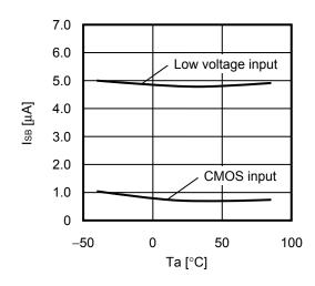
1. 14 Input leakage current I∟ vs. Ambient temperature Ta
