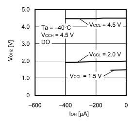
1. 25 High level output voltage V<sub>OH2</sub> vs. High level output current loh
