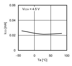
1. 9 Internal oscillator current consumption during operation I<sub>CC3</sub> 1. 10 Internal oscillator current consumption during operation I<sub>CC3</sub> vs. Ambient temperature Ta
