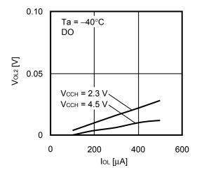
1. 23 Low level output voltage V<sub>OL2</sub> vs. Low level output current l<sub>OL</sub>
