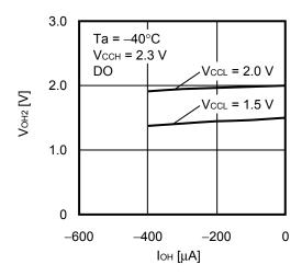
1. 27 High level output voltage V<sub>OH2</sub> vs. High level output current I<sub>OH</sub>
