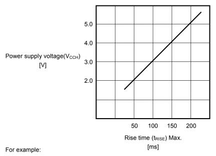
If your S-7760A's supply voltage = 3.0 V, raise the power supply voltage to 3.0 V within 100 ms.
