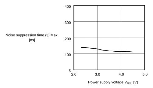
Figure 37 Noise Suppression Time for SDA and SCL Pins (CMOS input type)
