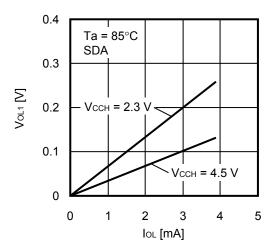
1. 22 Low level output voltage  $V_{\text{OL2}}$  vs. Low level output current  $I_{\text{OL}}$
