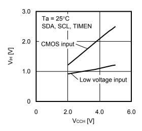
1. 31 High level input inversion voltage V<sub>IH</sub> vs. Ambient temperature Ta
