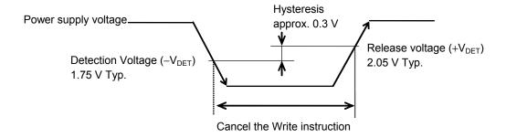
Figure 31 Operation during Low Power Voltage
