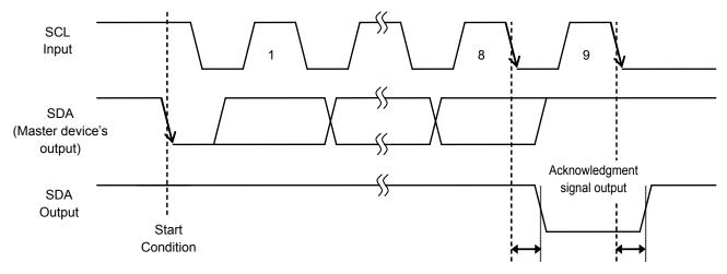
Figure 25 Acknowledgment Output Timing
