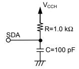
Figure 10 Output Load Circuit
