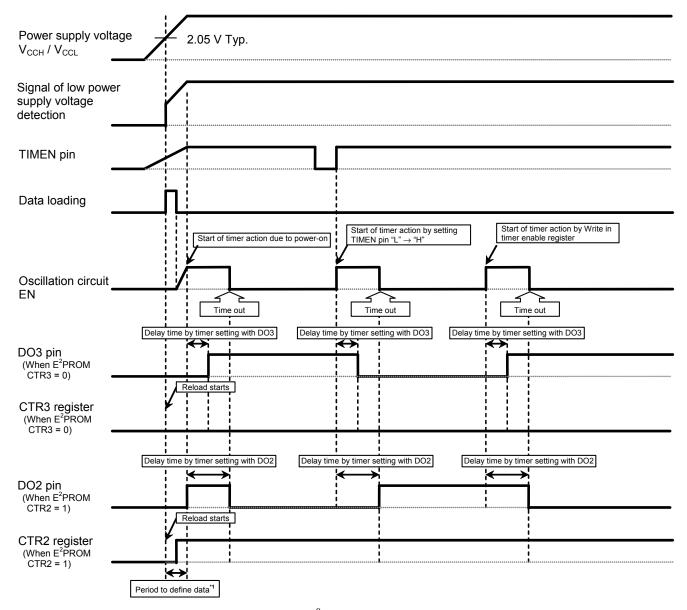
\*1. A period to define data is; the loading period from  $E^2PROM +$  the period to stabilize output from DO7 to 0 pin = within 100  $\mu$ s.
