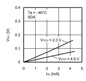
1. 19 Low level output voltage V<sub>OL1</sub> vs. Low level output current I<sub>OL</sub>
