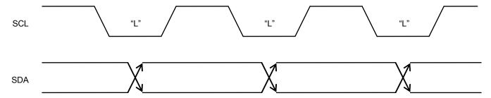
Figure 24 Data Transfer Timing
