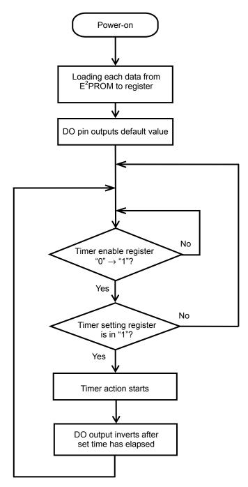
Figure 22 Flowchart of S-7760A's Action (When selecting "condition to start timer Option 2")
