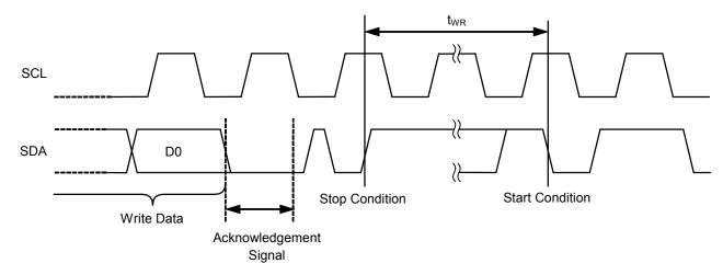
Figure 12 Write Cycle Timing
