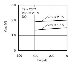
1. 29 High level output voltage V<sub>OH2</sub> vs. High level output current loh
