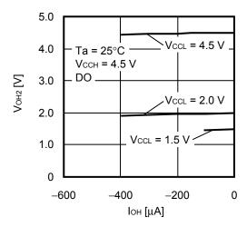
1. 28 High level output voltage V<sub>OH2</sub> vs. High level output current I<sub>OH</sub>
