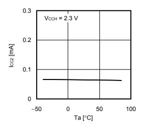
1. 8 Current consumption (PROGRAM) Icc2 vs. Power supply voltage Vcch
