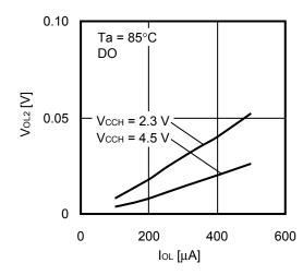
1. 20 Low level output voltage V<sub>OL1</sub> vs. Low level output current I<sub>OL</sub>
