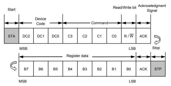
Figure 13 Device Address
