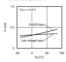
2. 6 SDA output delay time t<sub>AA</sub> vs. Ambient temperature Ta
