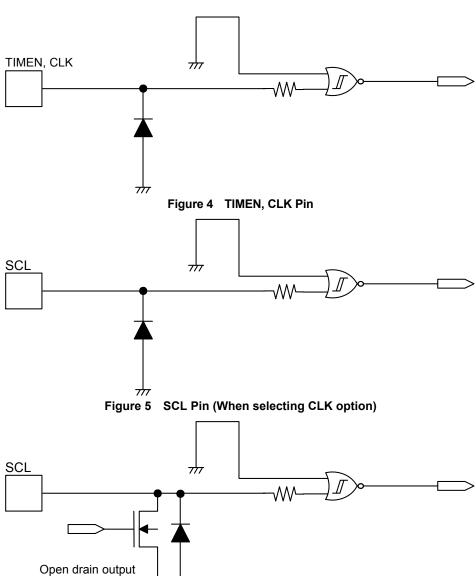
Figure 6 SCL Pin (When selecting BPDX option)
