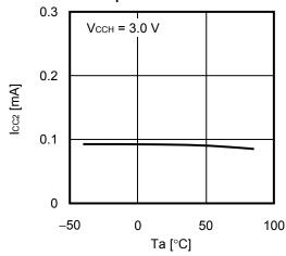
Current consumption (PROGRAM) Icc2 vs. Ambient temperature Ta
