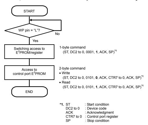
Figure 30 Flowchart for Software Example 2
