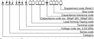
(Note1) : PSJ series,  $2.5V560\mu F$  (ESR 4m  $\Omega$  max.) has supplement code "J". Terminal and terminal plating are the same as all other in PSJ series.
