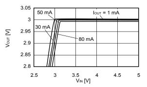
(3) Dropout voltage vs. Output current
