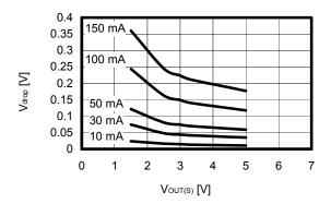
(4) Dropout voltage vs. Set output voltage
