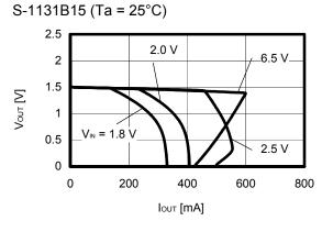
(1) Output voltage vs. Output current (when load current increases)
