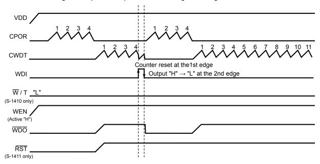
Figure 36 Double Pulse Detection
