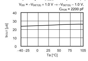
7. Watchdog output delay time ( $t_{WOUT}$ ) vs. Temperature (Ta)
