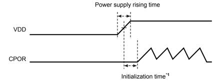
\*1. The initialization time is the time period from when the VDD pin voltage reaches VDD / 2 to when CPOR rises.
