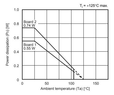
Figure 44 Power Dissipation of Package (When Mounted on Board)
