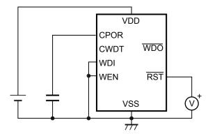
Figure 12 Test Circuit 5
