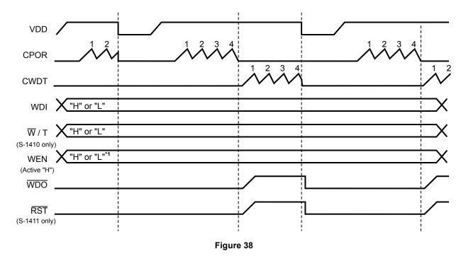
\*1. When the WEN pin is Disable, the charge-discharge operation of CWDT pin is not performed.
