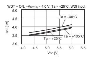
2. Current consumption during operation (I<sub>SS1</sub>) vs. Temperature (Ta) 3. Detection voltage (-V<sub>DET</sub>), Release voltage (+V<sub>DET</sub>) vs. Temperature (Ta)
