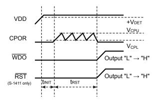
**Remark**  $V_{CPU}$ : CPOR charge upper limit threshold (1.25 V typ.)  $V_{CPL}$ : CPOR charge lower limit threshold (0.20 V typ.)
