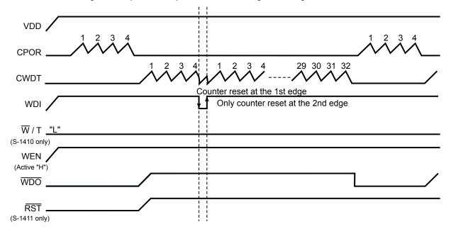
Figure 37 Double Pulse Non-detection
