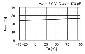
6. Reset output delay time (t<sub>ROUT</sub>) vs. Temperature (Ta)
