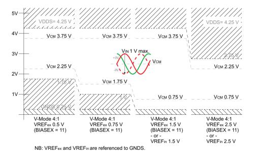
Figure 4: Permissible common mode range for voltage input 4:1 in dependancy to the reference voltage.
