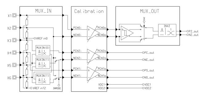
Figure 5: Multiplexer Schematics
