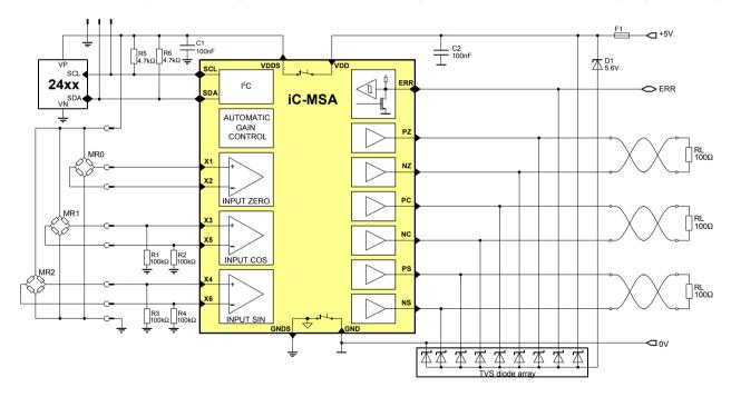
Figure 8: Example circuit for safety-related applications with iC-MSA.
