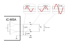
Figure 6: Definition of 1 Vpp signal. Termination R0 must be high-ohmic during all *Test* and *Calibration* modes.
