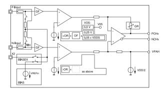
Figure 2: Signal conditioning input circuit.
