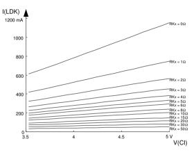
Figure 4: Diode current vs. V(CI) at Tj = 27 °C
