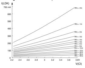
Figure 3: Diode current vs. V(CI) at Tj = 27 °C
