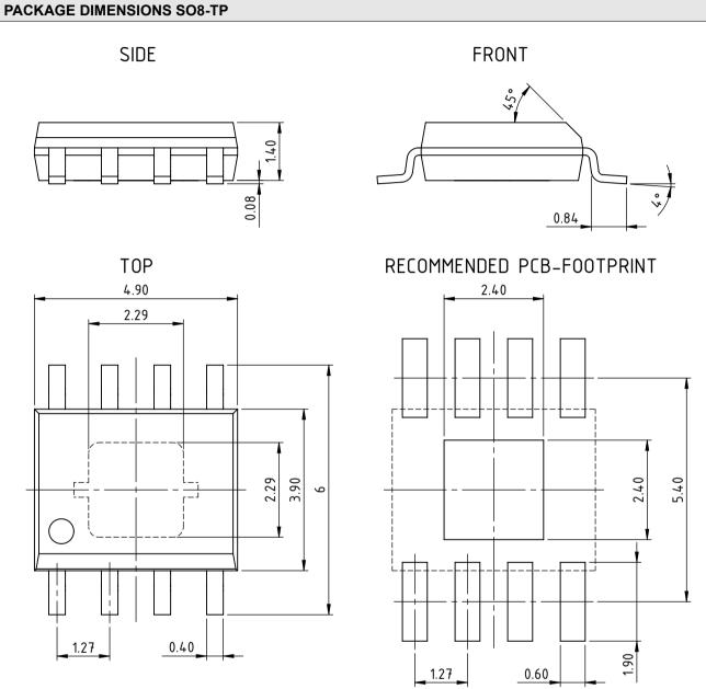
All dimensions given in mm. Tolerances of form and position according to JEDEC MS-012 dra\_so8-tp-3\_pack\_1, 10:1
