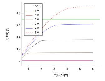
Figure 7: Output Characteristics of LDK
