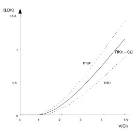
Figure 6: Diode current variation vs. V(CI) at V(LDK) = 3 V
