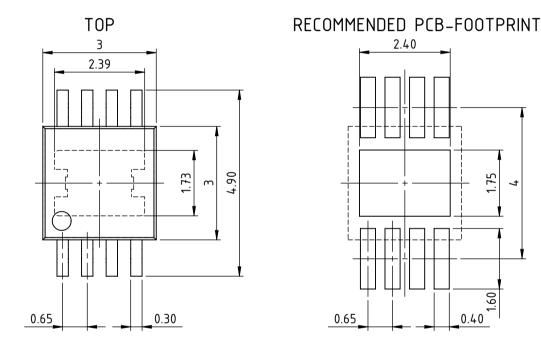
All dimensions given in mm. Tolerances of form and position according to JEDEC MO-187. dra\_msop8-tp-1\_pack\_1, 10:1
