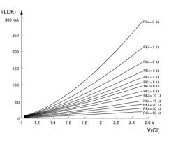
Figure 2: Diode current vs. V(CI) at Tj = 27 °C
