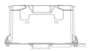
Even though the ground connects correctly through the DIN rail, may not get noise attenuation. Be sure to connect the FG ground of EMI filter to the ground directory.
