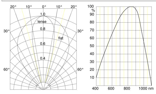
Figure 1: Directional characteristics  $S_{rel}(\phi)$
