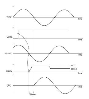
Figure 8: Utilising the SYNC input
