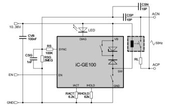
Figure 7: Utilising the SYNC input
