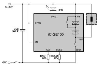
Figure 3: Activation by switching GND
