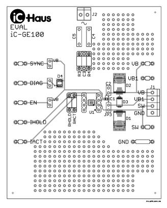
Figure 10: Evaluation board (component side)
