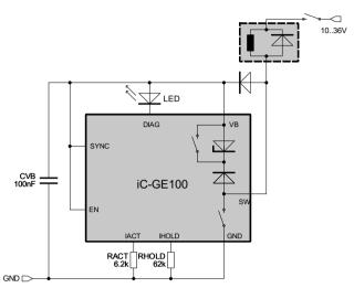
Figure 6: Low-side driver for relays with free-wheeling diode
