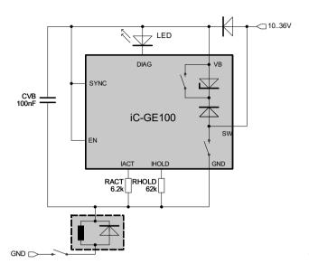
Figure 5: High-side driver for relays with free-wheeling diode
