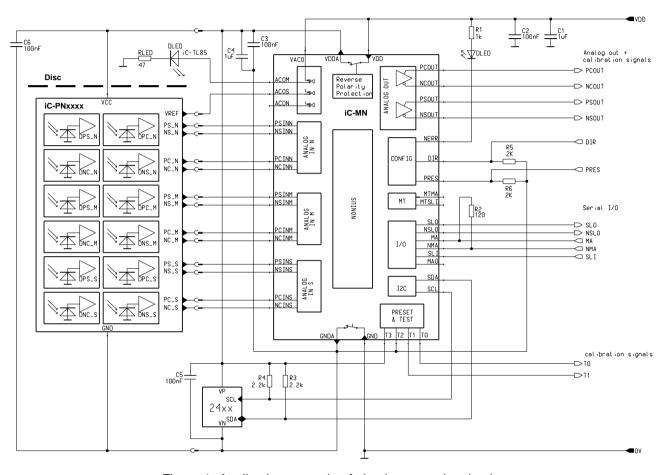
Figure 1: Application example of absolute encoder circuit.
