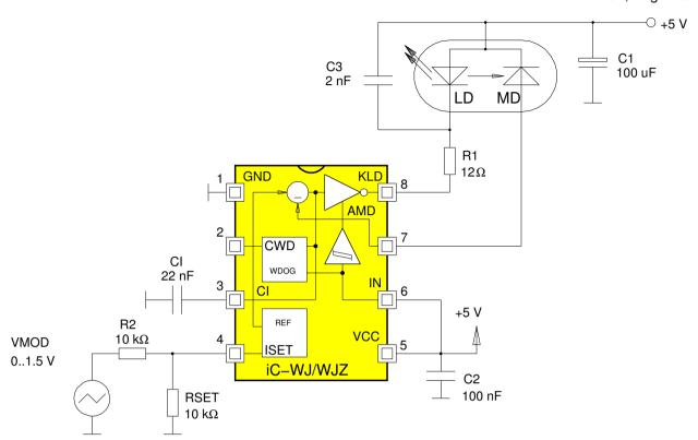
Figure 11: Analogue modulation during CW operation
