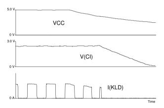
Figure 7: Turn-off behavior, f(IN) = 100 kHz (1:1), CI = 470 nF, RSET = 10 k $\Omega$
