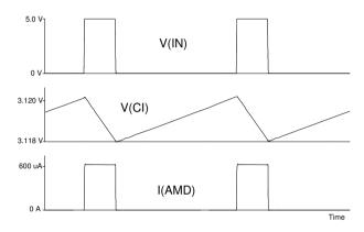
Figure 4: Steady-state averaging, f(IN) = 100 kHz(1:4), CI = 470 nF,  $RSET = 10 \text{ k}\Omega$
