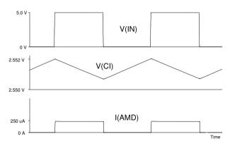
Figure 3: Steady-state averaging control, f(IN) = 100 kHz (1:1), CI = 470 nF, RSET =  $10 \text{ k}\Omega$
