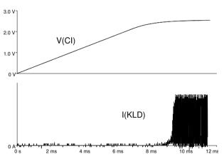
Figure 5: Turn-on behavior, f(IN) = 100 kHz (1:1), CI = 470 nF, RSET = 10 k $\Omega$
