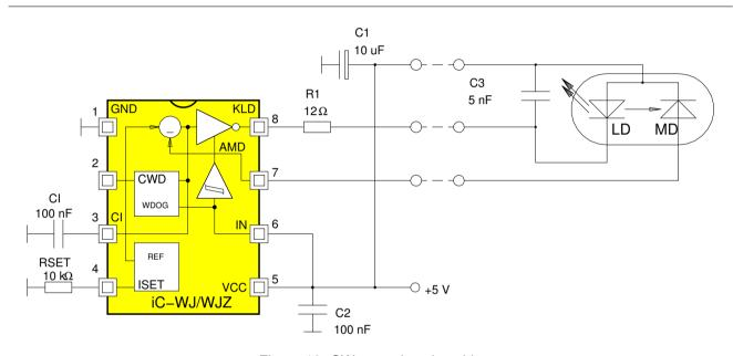
Figure 10: CW operation via cable
