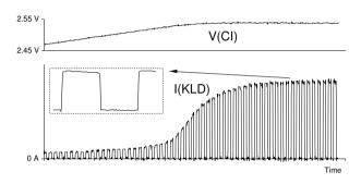
Figure 6: Turn-on behavior, detailed view f(IN) = 100 kHz (1:1), CI = 470 nF,  $RSET = 10 \text{ k}\Omega$
