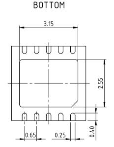
All dimensions given in mm. Tolerances of form and position according to JEDEC M0-229. Tolerance of sensor pattern: ±0.10mm / ±1° (with respect to center of backside pad). dra\_cdfn10-4x4-2\_lfs\_0\_pack\_1, 10:1
