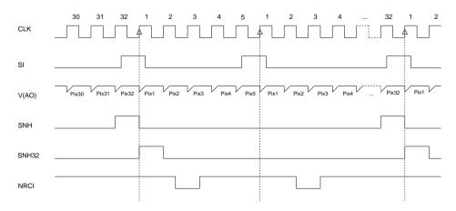
Figure 5: Restarting a readout cycle
