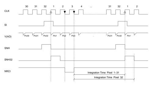
Figure 4: Readout cycle and integration sequence
