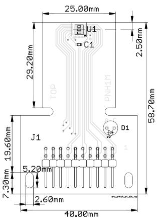
Figure 1: Sensor board PNH1M (top view)
