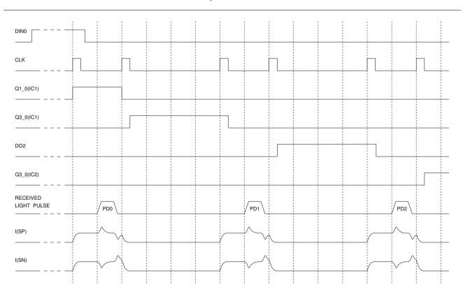
Figure 9: Signals for the chain configuration of Fig. 8
