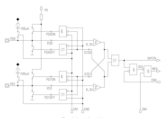
Figure 5: Input safety switch
