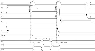
Figure 3: Differential output current pulse at SP and SN versus input current pulse at PD
