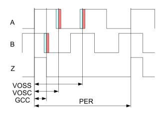
Figure 20: Calibration using incremental signals
