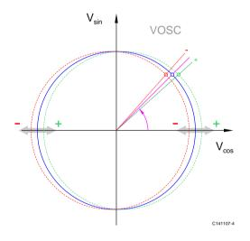
Figure 18: Effect of the cosine offset setting
