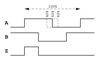
Figure 21: ABZ signals and relative accuracy
