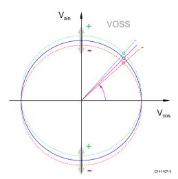
Figure 17: Effect of the sine offset setting
