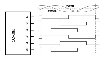
Figure 25: UVW differential commutation signals
