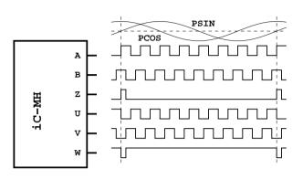
Figure 23: ABZ differential incremental signals
