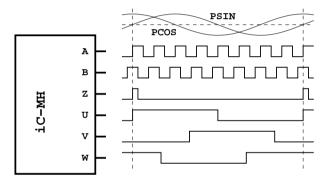
Figure 24: ABZ incremental / UVW commutation signals
