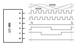
Figure 26: ABZ incremental signals / period counter
