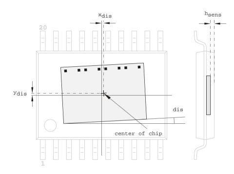
Figure 3: Definiton of lateral and rotational displacements
