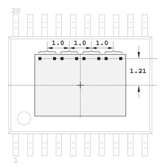
Figure 2: Hall sensor array of four sensor pairs spaced 1mm apart.
