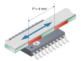
Figure 5: Typical arrangement of a magnetic tape to iC-MHL200
