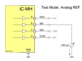
Figure 14: Setting bias current IBM in test mode Analog REF
