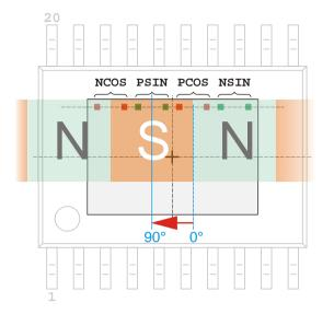
Figure 9: Position of the magnetic target at 90° electrical position. Center of south pole is aligned to the PSIN sensor pair
