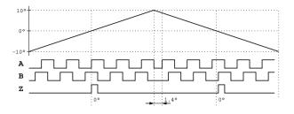
Figure 22: Quadrature signals for rotating direction reversal (hysteresis 1.4°)
