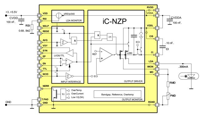
Figure 7: Example set-up for current control
