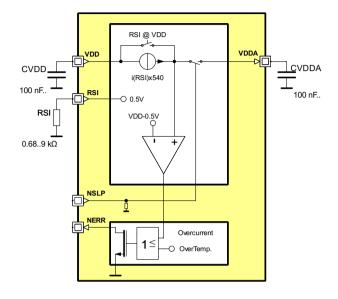
iC-NZP monitors the average laser current flowing from pin VDDA (Figure 6). The DC current limit is set by means of a resistor at pin RSI.
