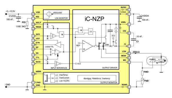
Figure 5: Circuit example for N-type laser diodes
