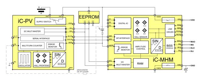
Figure 12: Application example iC-PV as battery-buffered multiturn device connected to the MT interface of the iC-MHM singleturn encoder. Interface operating in SSI-Mode (INT\_MODE = 0). The two iC's share one common EEPROM for configuration. EEPROM is written via iC-MHM, BiSS register access. The position (MT + ST) is transmitted via the serial BiSS interface (please see iC-MHM specification for further details).
