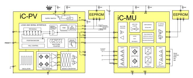
Figure 13: Application example iC-PV as battery-buffered multiturn device connected to the MT interface of the iC-MU absolute singleturn encoder. Interface operating in SSI-Mode (INT\_MODE = 0). One EEPROM per iC mandatory for configuration. iC-PV EEPROM, direct access via SCL, SDA. BiSS, SPI and SSI are available for serial data transmission (please see iC-MU specification for further details).
