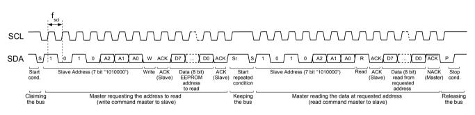
Figure 11: iC-PV combined write/read command reading one slave address.
