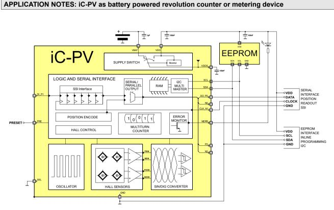
Figure 17: Application example iC-PV as battery powered multiturn counter, e.g. in a metering application. Interface operating in SSI-Mode (INT\_MODE = 0) is used to readout the internal counter value. iC-PV is battery powered. VDD Supply is only needed during readout. EEPROM programming inline over SCL/SDA.
