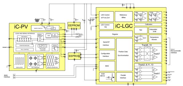
Figure 14: Application example iC-PV as battery-buffered multiturn device connected to the MT interface of the iC-LGC optical singleturn encoder. Interface operating in SSI-Mode (INT\_MODE = 0). One EEPROM per iC mandatory for configuration. iC-PV EEPROM, direct access via SCL, SDA. BiSS, SPI and SSI are available for serial data transmission (please see iC-LGC specification for further details).
