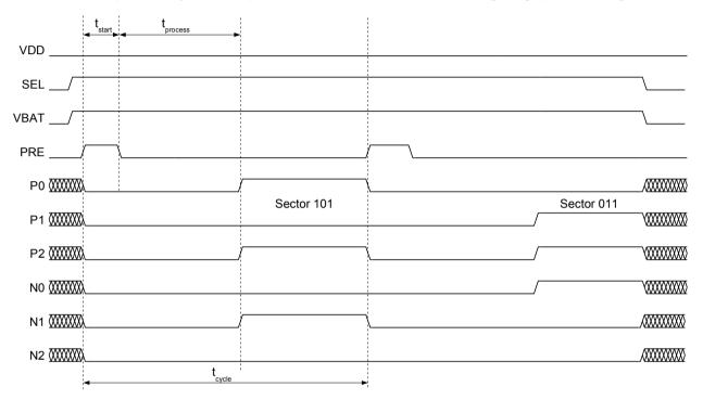
Figure 10: Line signals for parallel mode (3 bit complementary P0-P2 and N0-N2).
