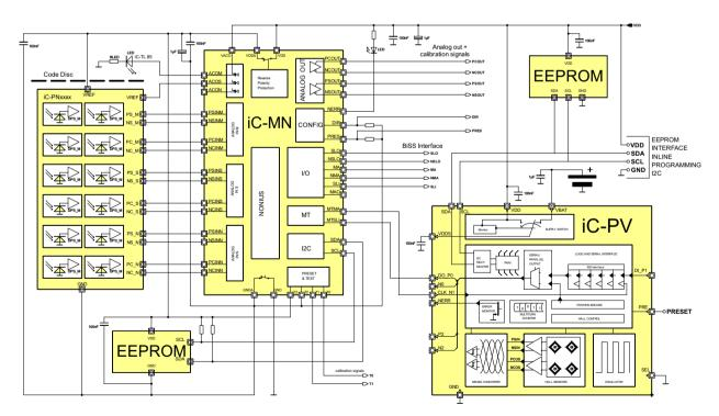
Figure 15: Application example iC-PV as battery-buffered multiturn device connected to the MT interface of the iC-MN nonius encoder (together with an iC-PN type phased array). iC-PV Interface operating in SSI-Mode (INT\_MODE = 0). One EEPROM per iC mandatory for configuration. iC-PV EEPROM, direct access via SCL, SDA. BiSS or SSI are available for serial data transmission (please see iC-MN/PNxxxx specification for further details).
