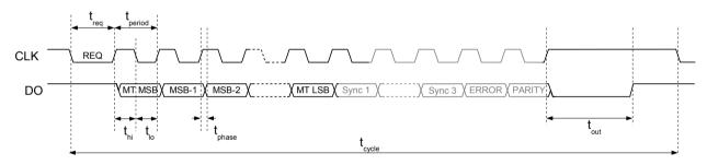
Figure 8: I/O line signals of the serial interface in SSI mode (INT\_MODE = 0).
