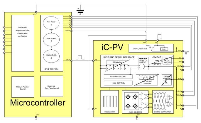
Figure 18: Application example of iC-PV acting as parallel mode (3 bit). All intelligence (counting, spike control and period selection etc.) is provided by the mandatory microcontroller in this arrangement. Hence, the crossed-out blocks are not used in this operating mode.
