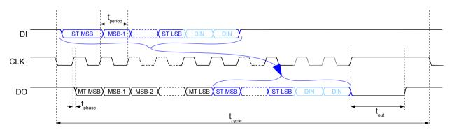
Figure 9: I/O line signals of the serial interface in chain mode (INT\_MODE = 1).
