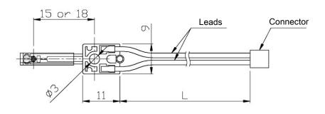
Features: A high speed type temperature sensor that can guickly respond to
