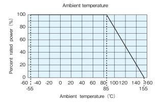
For resistors operated at an ambient temperature of  $85^\circ\!\!\mathrm{C}$  or higher, the power shall be derated in accordance with the above derating curve.
