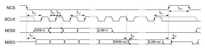
Figure 3: SPI Access
