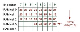
Figure 6: Example Frame in RAM
