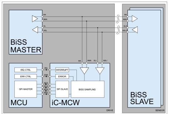
Figure 1: Integration of the iC-MCW in a BiSS Communication System
