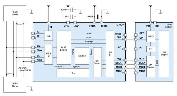
Figure 4: Connections of the iC-MCW
