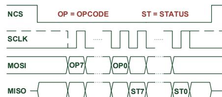
Figure 8: SPI Transmission ReadStatus
