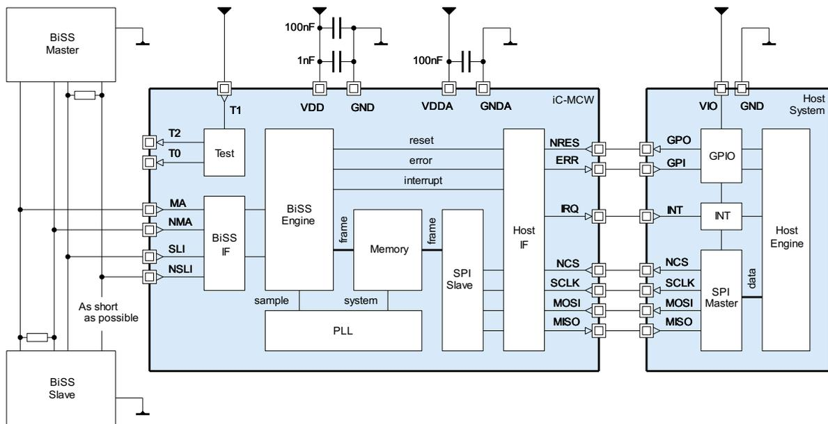
Figure 4: Connections of the iC-MCW
