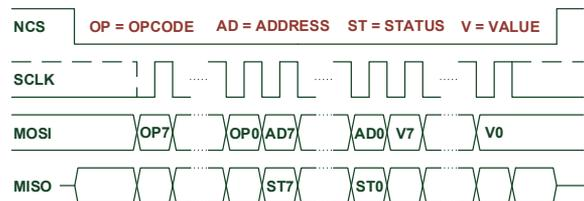
Figure 12: SPI Transmission WriteRegister
