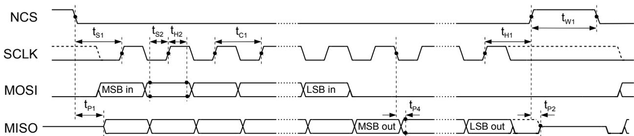
Figure 3: SPI Access
