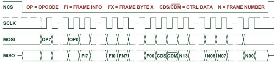
Figure 10: SPI Transmission ReadFrameData
