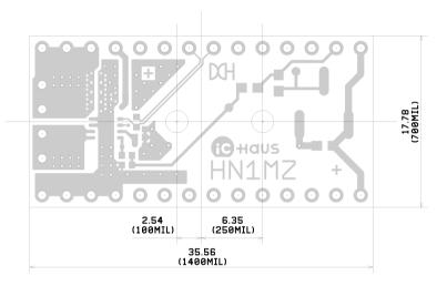
Figure 2: Top view / Dimensions in mm
