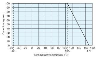
When the terminal part temperature of the jumper exceeds the rated terminal part temperature shown above, the power shall be derated according to the derating curve.
