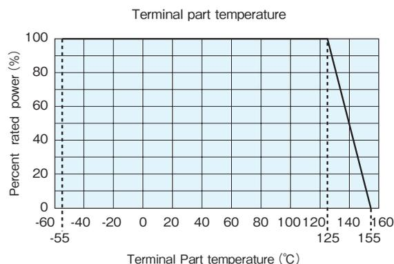
For resistors operated at an ambient temperature of 85°C or higher, the power shall be derated in accordance with the above derating curve.
