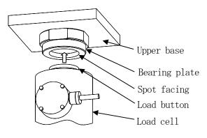
• The construction of bearing plate has made so that the bearing plate will be screwed to the upper base. This is the reason to put the shim plate between the upper base and bearing plate for the purpose of level adjustment. Use the bearing plate with fully screwed up.
