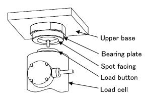
• The construction of bearing plate has made so that the bearing plate will be screwed to the upper base. This is the reason to put the shim plate between the upper base and bearing plate for the purpose of level adjustment. Use the bearing plate with fully screwed up.
