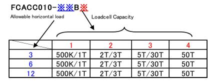
Note: Depending on the capacity of load cell applied, the corresponding form shall differ. When you request the installing metals, specify the capacity of load cell (P/N) together with them.
