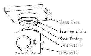
• The construction of bearing plate has made so that the bearing plate will be screwed to the upper base. This is the reason to put the shim plate between the upper base and bearing plate for the purpose of level adjustment. Use the bearing plate with fully screwed up.
