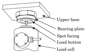
• The construction of bearing plate has made so that the bearing plate will be screwed to the upper base. This is the reason to put the shim plate between the upper base and bearing plate for the purpose of level adjustment. Use the bearing plate with fully screwed up. Never use the bearing plate with some space between the bearing plate and upper base, or never use the bearing plate instead of a jack.
