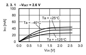
2.4 Reset output current vs. Output voltage
