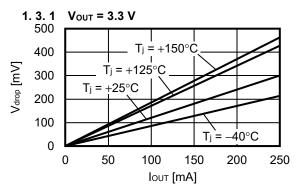
1.4 Dropout voltage vs. Junction temperature
