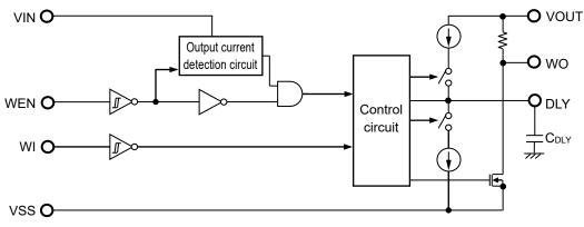
Figure 26 Operation of Watchdog Timer Block
