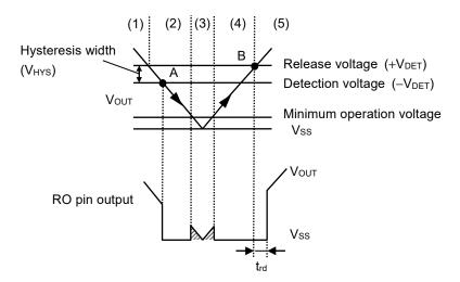
Figure 23 Timing Chart of Detector Block
