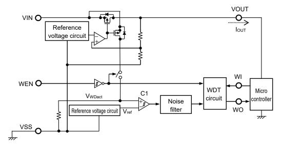
Figure 27 Operation of Output Current Detection Circuit
