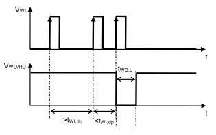
Figure 8 Watchdog Double-pulse Detection Time
