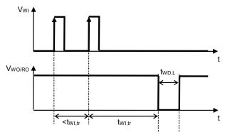
Figure 7 Watchdog Trigger Time
