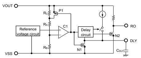
Figure 22 Operation of Detector Block
