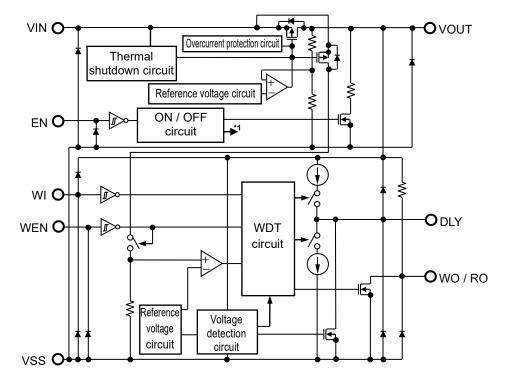
\*1. The ON / OFF circuit controls the internal circuit and the output transistor.
