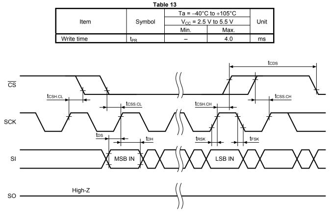
Figure 4 Serial Input Timing
