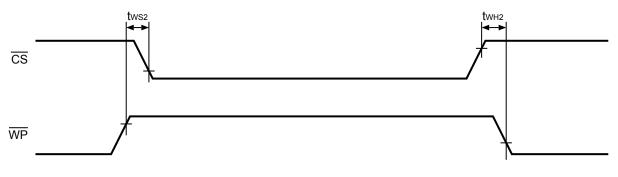
Figure 8 Invalid Timing in Write Protect
