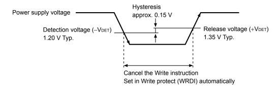
Figure 19 Operation during Low Power Supply Voltage
