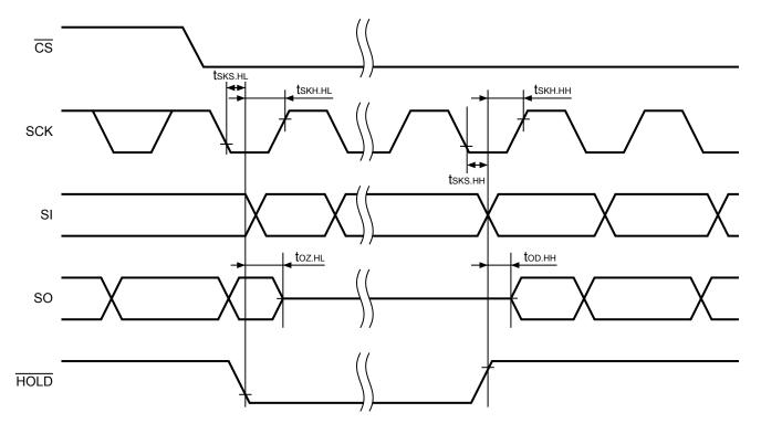
Figure 6 Hold Timing ABLIC Inc.
