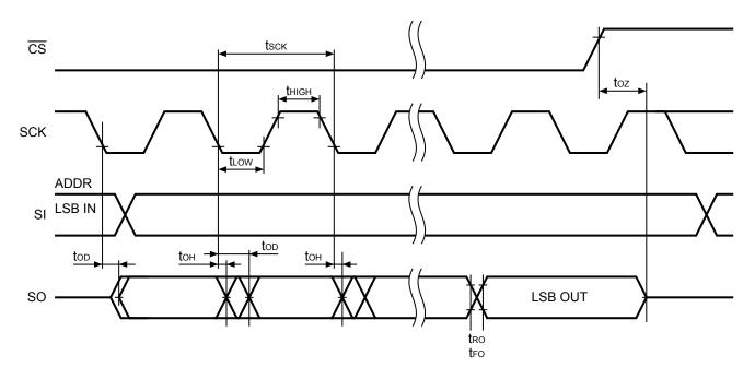
Figure 7 Serial Output Timing
