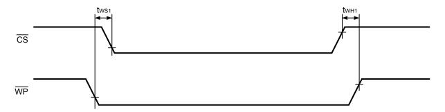
Figure 8 Valid Timing in Write Protect
