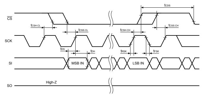
Figure 5 Serial Input Timing
