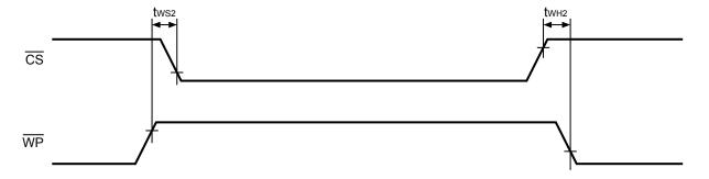
Figure 9 Invalid Timing in Write Protect
