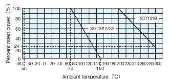
For sensors operated at an ambient temperature or higher, the power shall be derated in accordance with the above derating curve.
