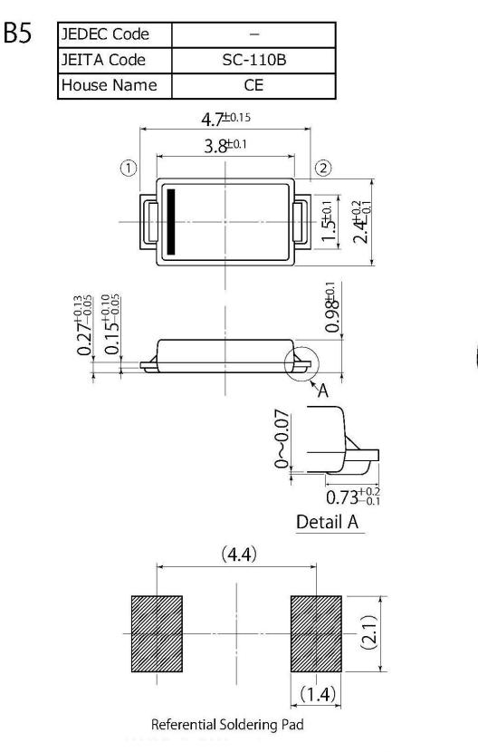
• Optimize soldering pad to the board design and soldering condition.
